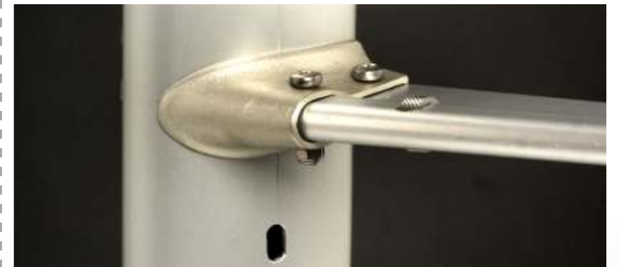
Saling, justerbar for let justering af mast kurve.
